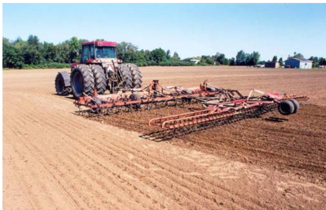
Small tooth cultivator with homebuilt rake at rear.
