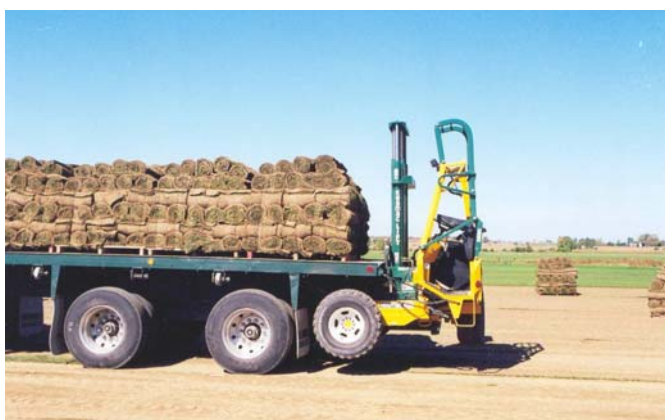
Kesmac Truckmounted Forklift goes with the load of sod to unload it at the customer's location.
