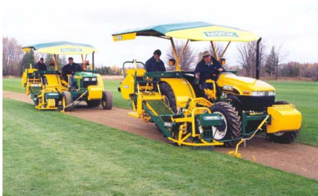
Kesmac 2150 Harvesters for Roll or Slab Harvesting with Unique Pivoting Conveyor /Cutter Head.
