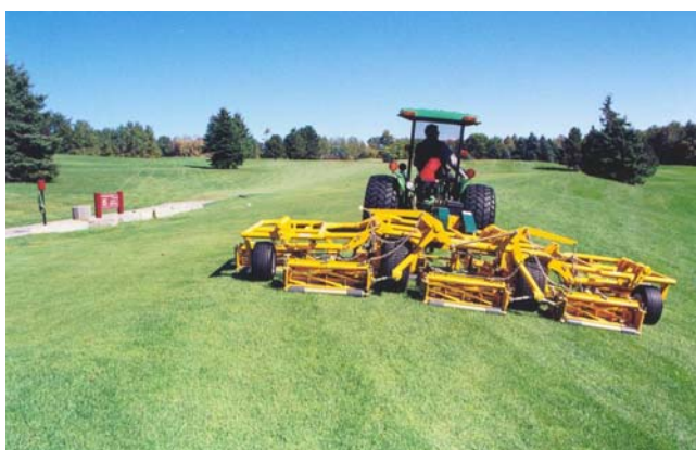
Kesmac Fairway Mowers have a floating head design allowing them to follow ground contours. Easily pulled by a lightweight low hp. tractor.
