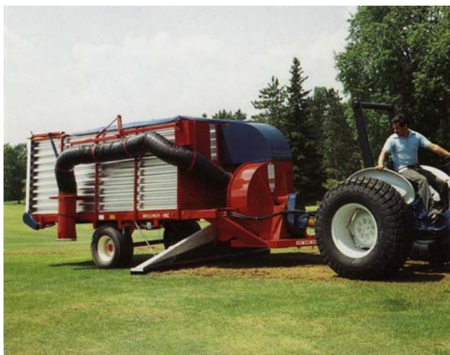
Vacuum picks up clippings and debris from turf.
