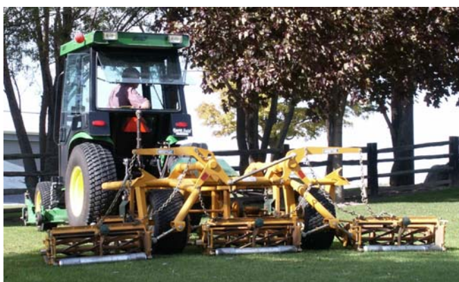
5 Gang configurations with cutting widths up to 25 feet.
