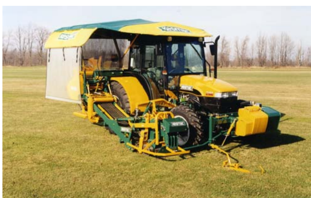
Available options include 2 or 4 wheel drive, fully equipped cab and weather protection for stackers.
