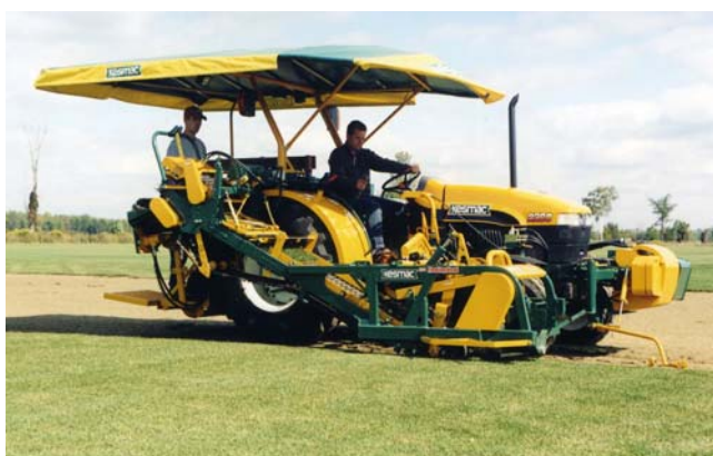
Kesmac 2200 Sod Harvester with Full Floating Head for Roll or Slab Harvesting.
