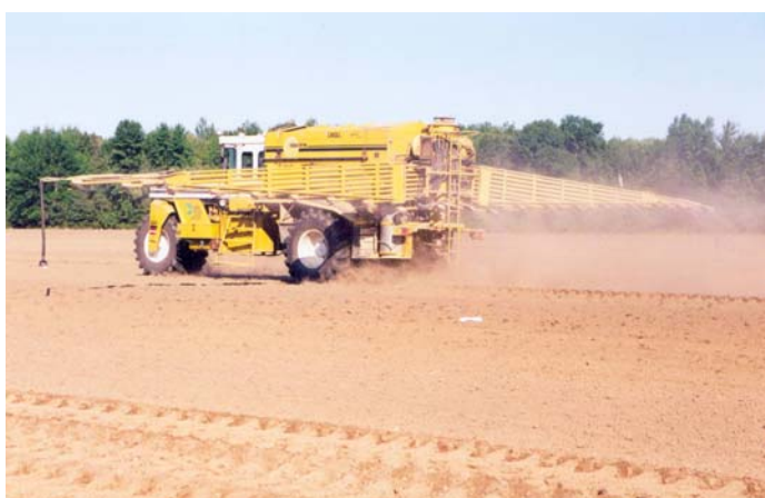
Large volume machine to apply fertilizer before seeding.
