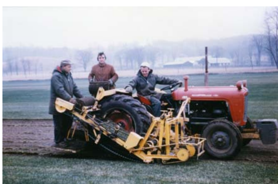
This was the second Harvester Gerry made in July 1966. Much simpler, PTO and V-Belt Drive still needed a three man crew.
