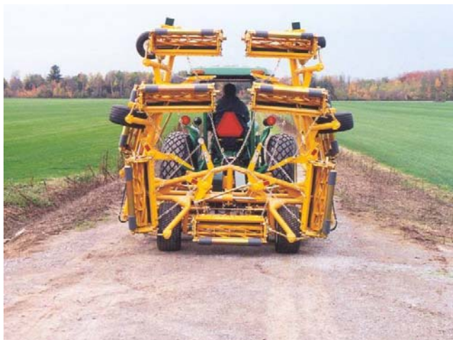
Kesmac 11 Gang Reel Mower in transport position, is easily moved from field to field.
