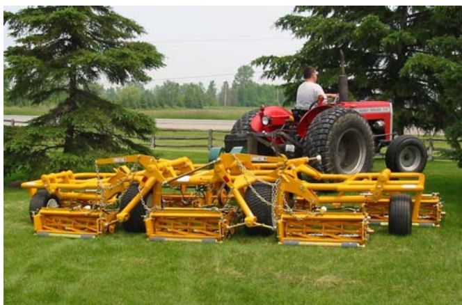
7 Gang configurations with cutting widths up to 25 feet.
