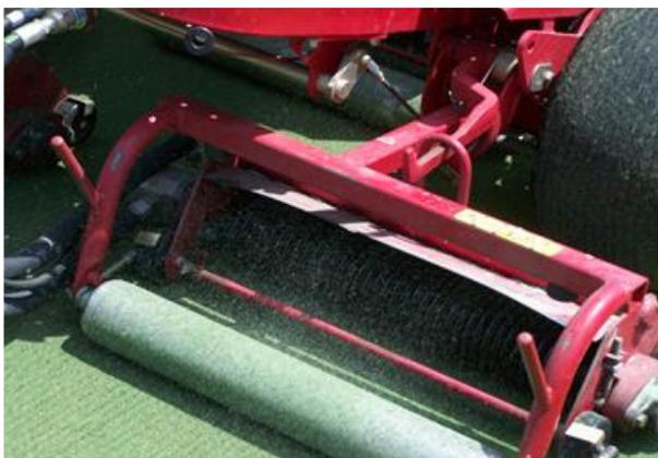
**Fig 34.** Light verta-cutting with riding mower (many times down and back).
